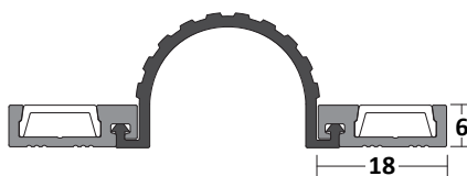
Lorient Finger Guards Rear (measurements in mm)
